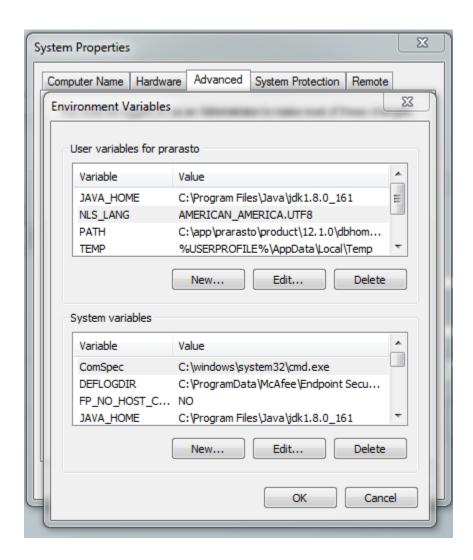
After this, go to Run(shortcut:Windows+R), enter regedit, and click OK. It will open Registry Editor. Here, under Oracle DB KEY, NLS\_LANG parameter can be added with variable name as NLS\_LANG and value as AMERICAN\_AMERICA.UTF8 as shown in below picture.
